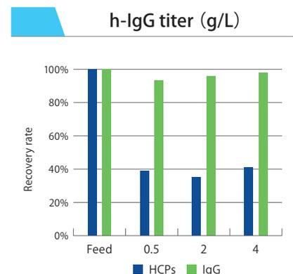
Condition : Feed CHO-K1 after clarification, HCPs 200 µg/mL, ratio 1/20, contact time 5 min
